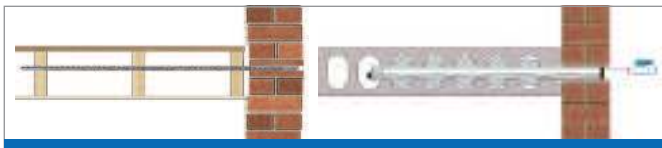
5 Stabilising bowed or disconnected walls into floors
