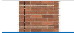
3 Repairing cracks near corners and openings
