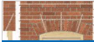
2 Repairing brick arch lintels
