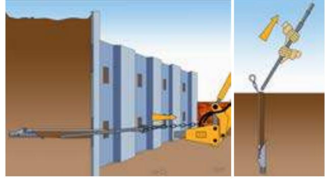
Once the anchor has been driven to the required depth the drive rod is removed for reuse.
