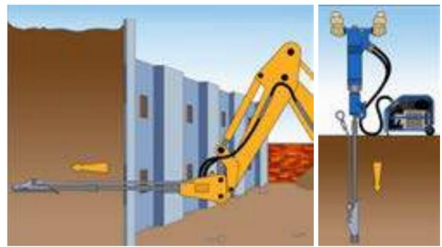
Vulcan anchors are designed to be driven into the ground using hydraulic or percussion equipment, with little or no disruption to the structure or surrounding area.
