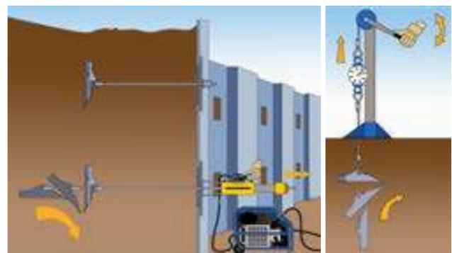
A tensile load is applied to the attached tie bar or tendon. This rotates the anchor into the locked position for maximum load holding capacity. The anchor is then proof tested to the designed loading requirements before the top termination is fitted, as specified by the civil or structural engineer.
